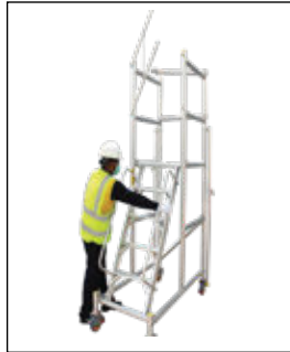
STEP-3 Fit inclined ladder On 3rd rung from top to the podium lower rungs. As per this picture
