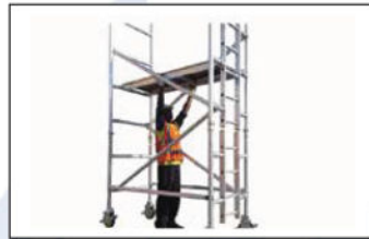
Step 7 Position trapdoor platform on 3rd rungs from the top Make sure the trapdoor opens to the ladder side. Engage windlock. (As ILLUSTRATION 3)
